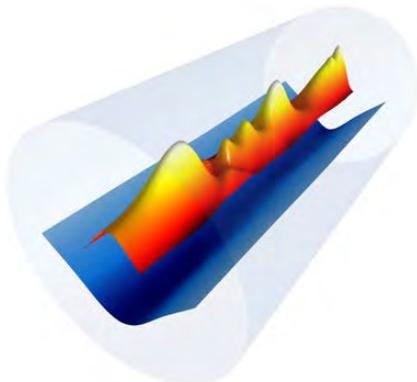
Plasma channel's electron density profile (blue) formed by discharge inside a capillary (gray) with an 8-nanosecond laser pulse heater (red, orange, and yellow). The plasma channel was used to guide femtoseconds-long "driver" laser pulses from the BELLA petawatt laser system, which generated plasma wake waves accelerating electrons to 8 GeV over the distance of 20 centimeters.
