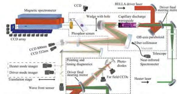
Layout of the BELLA LPA with laser heater for enhancing the capillary discharge waveguide
